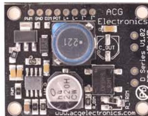
D1000 1000mA constant current AC/DC input
