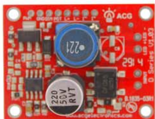
D350 350mA constant current AC/DC input
