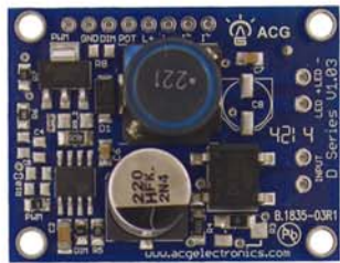
D700 700mA constant current AC/DC input
