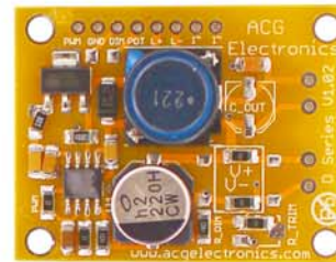
D1400 1400mA constant current DC input only
